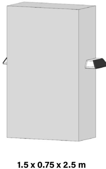
Figure 10: Top-deck payload: Overall dimensions of payload design envelope.
