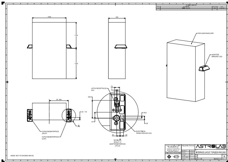
Figure 18: Top-deck payload and interface specification. [\(Click to download\)](#)
