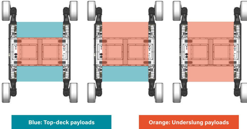
Figure 8: Top-view illustration of select FLEX payload configurations.
