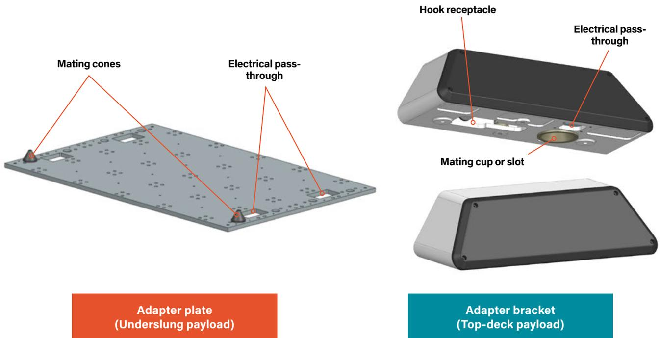
**Figure 17:** Mechanical adapters for underslung payload (left) and top-deck payload (right).
