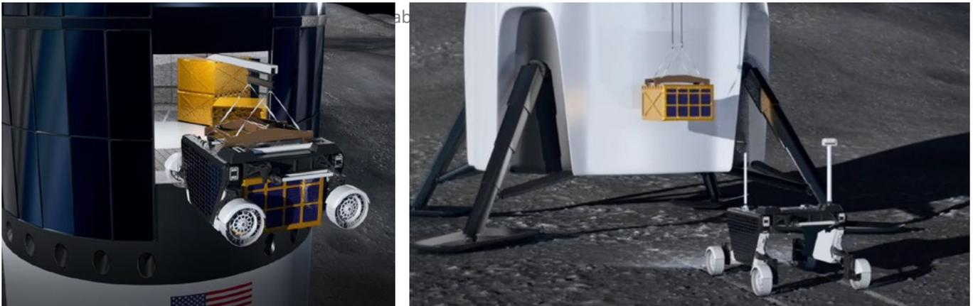
**Figure 2:** The Astrolab intermodal payload standard provides the ability for a single lander to deliver many payloads that a FLEX rover can transport.
