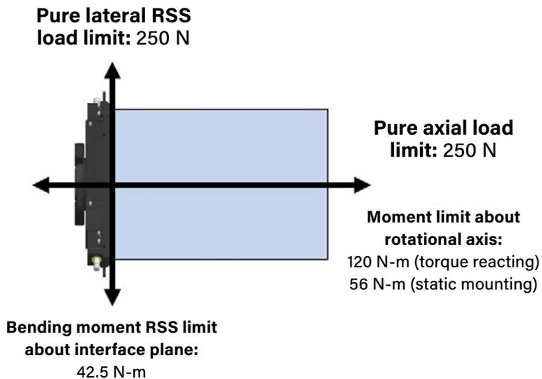
Figure 16: Robotic arm load limits for preliminary design.
