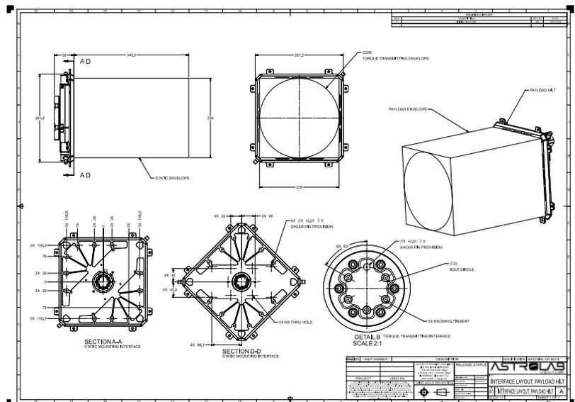
Figure 20: Robotic arm payload adapter specification. [\(Click to download\)](#)
