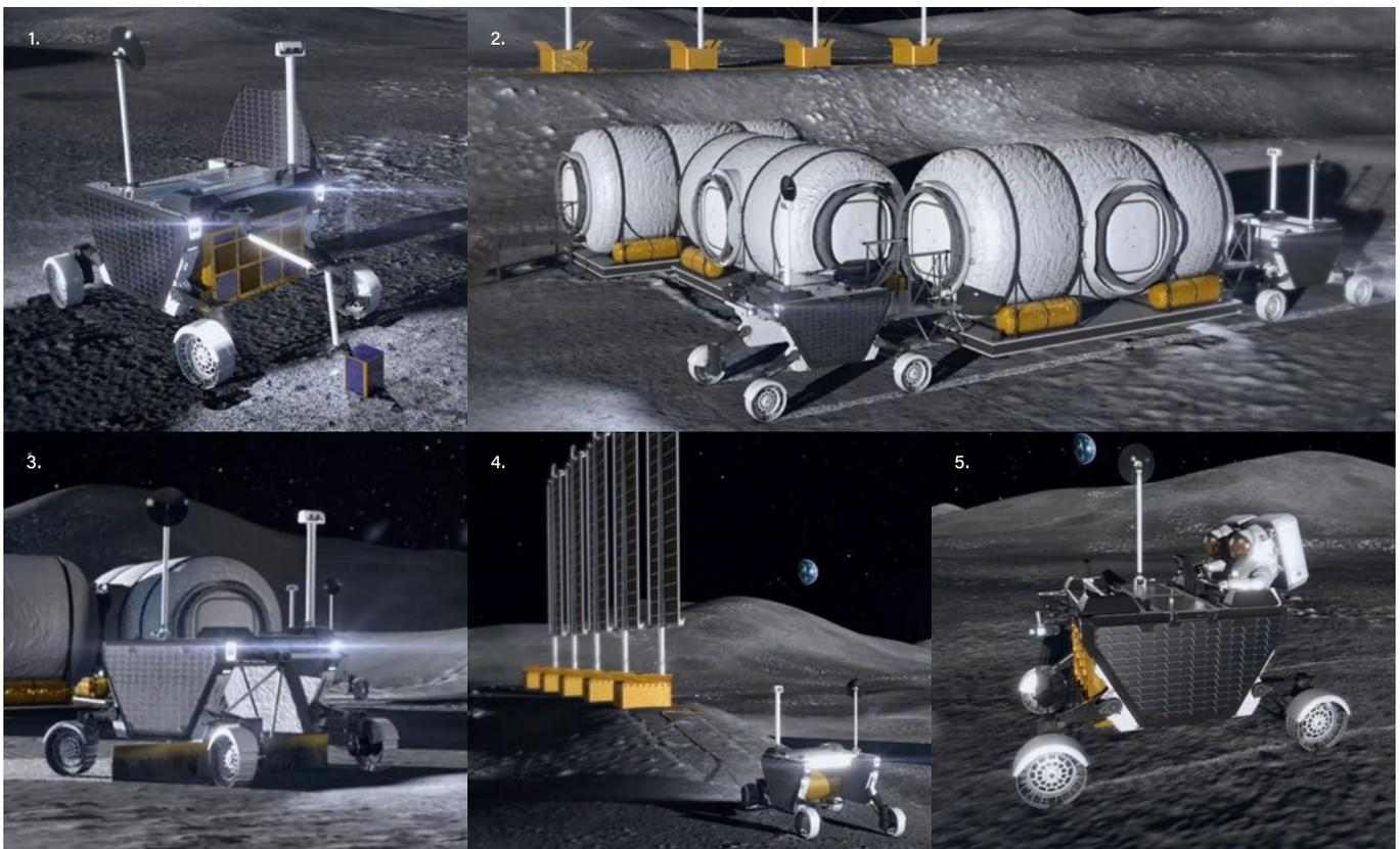
**Figure 3:** FLEX's modular payload interface and novel mobility system enable it to perform a multitude of functions, including 1. Distributed science; 2. Coordinated multi-rover manipulation of large payloads to support outpost construction; 3. Regolith grading and excavation; 4. Surface power and transmission cable deployment; and 5. Crew transport and exploration.
