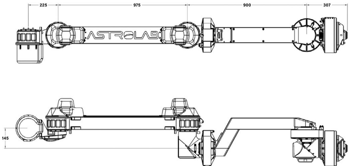
**Figure 6:** FLEX robotic arm dimensional layout.
