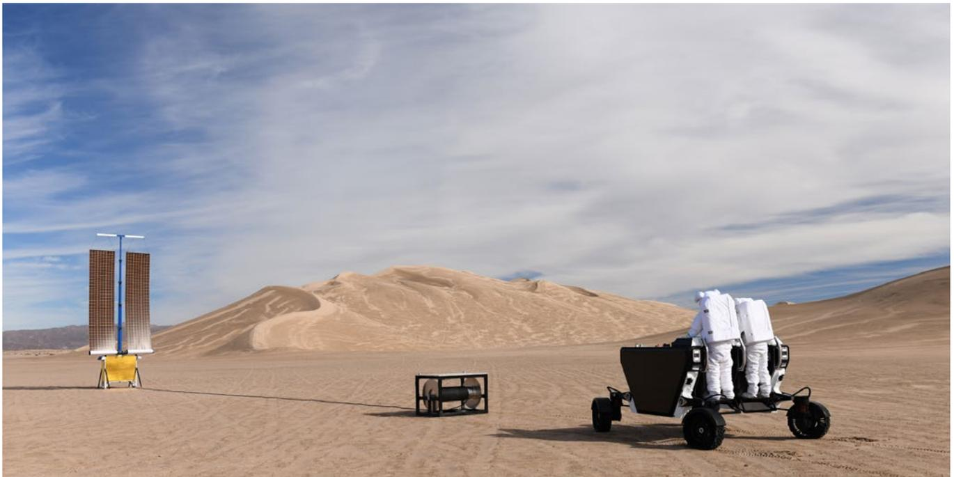
Figure 12: Field test deployment of a vertical solar array tower (a top-deck payload) and cable spool (an underslung payload). The rover's removable crew interface is another example of a top-deck payload.
