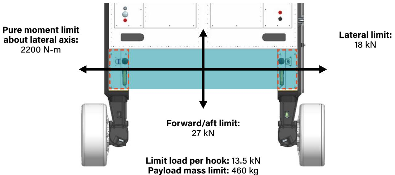
Figure 14: Top deck payload interface design limits.
