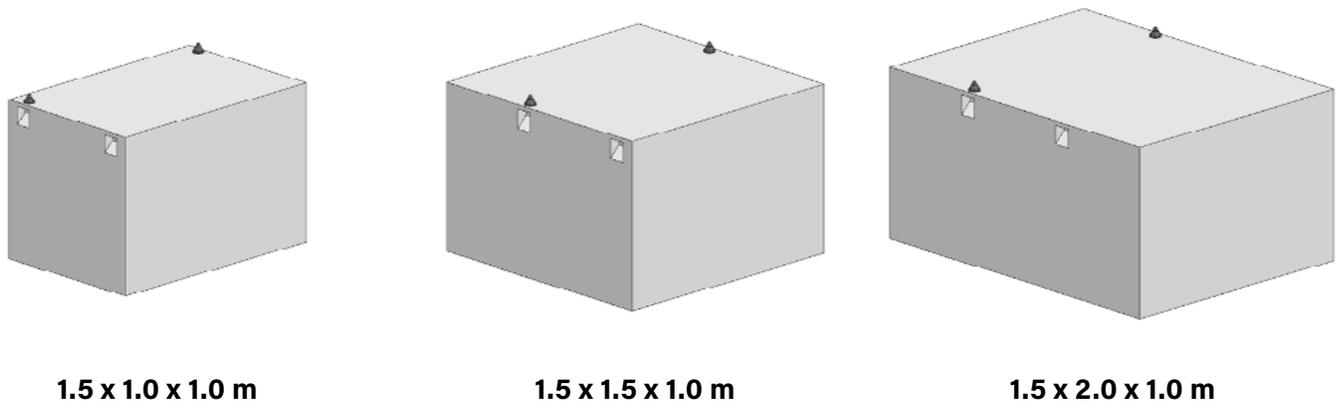
Figure 9: Underslung payloads: Overall dimensions of standard-size cargo containers.
