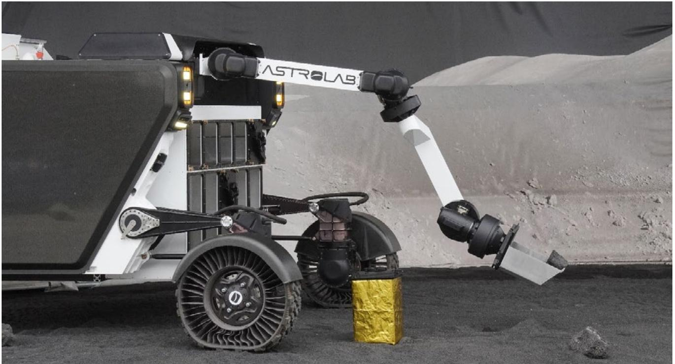
**Figure 5:** FLEX's 2m robotic arm has a modular end effector to add extensive functionality to the vehicle. The assembly is shown above with a sample collection scoop configuration after deployment of a payload with a 12U cubesat form factor.
