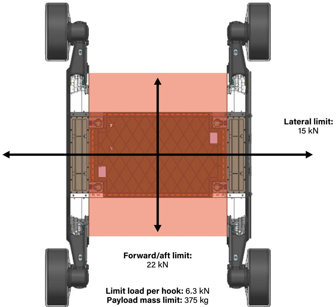
Figure 15: Underslung payload interface design limits.
